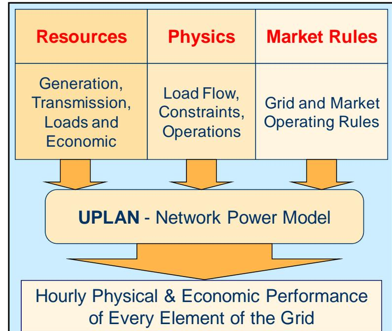
**UPLAN enables a detailed, granular simulation of market dynamics based on characterization of generators and the transmission network along with realistic representation of market protocols.**
