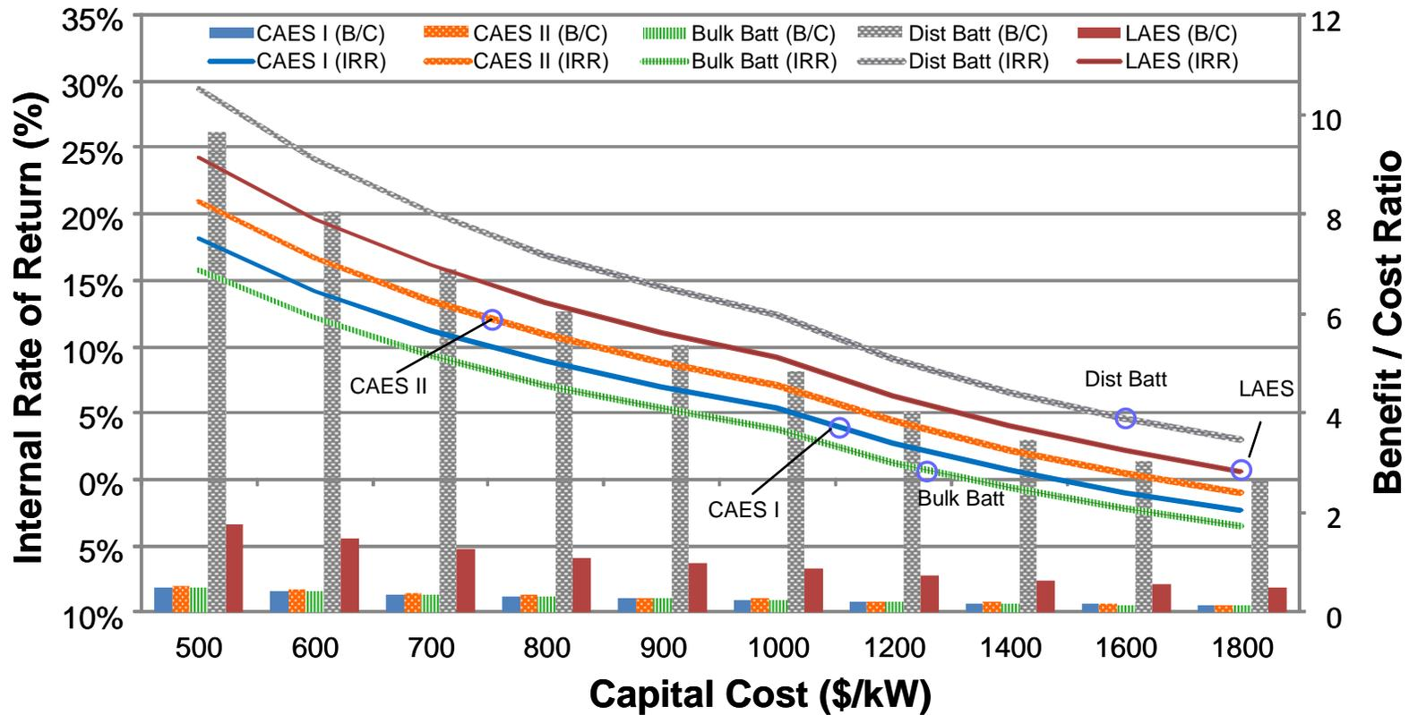
The 2009 study examined the role and value of CAES, bulk Battery, Distributed Battery ( Dist Batt) and Liquid Air energy Storage Systems (LAES)
